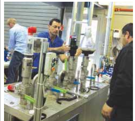
The A.R.I. air flow lab tests all types of air valves, including those with diameters from 1.2 to 30.48 cm (1/2 to 12 in).
