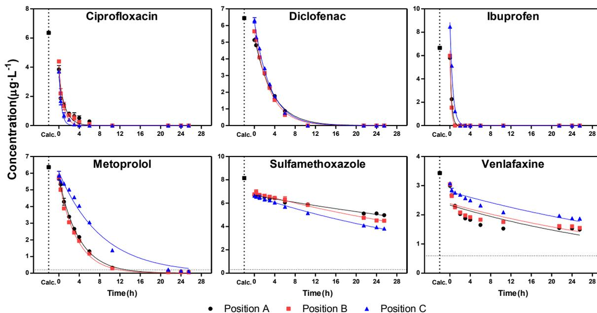
**Figure 19. Concentrations of selected pharmaceuticals during spiking experiment showing potential removal capacity in each reactor (Position A, B and C). Filled lines correspond to a first-order kinetics fitting. Black squares represent the theoretical concentration of individual pharmaceuticals based on stock solutions, (due to analytical complications, e.g. a shift in the retention time, clarithromycin and lomeprol were left out).**
