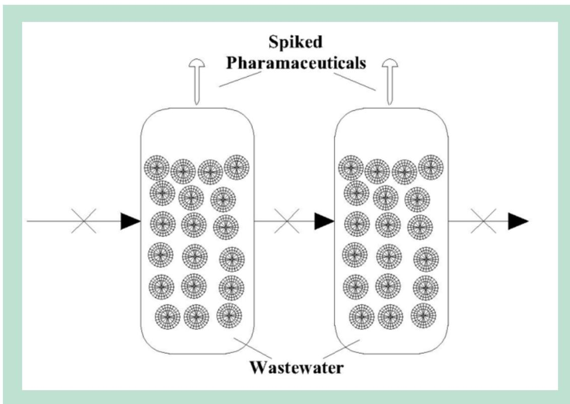
**Figure 5. Overview of the experimental setup for determining the potential capacity of the treatment technology, investigated in batch scale. The flow between reactors is discontinued while concentrations of spiked pharmaceuticals were measured over a 24 hour time-period.**
