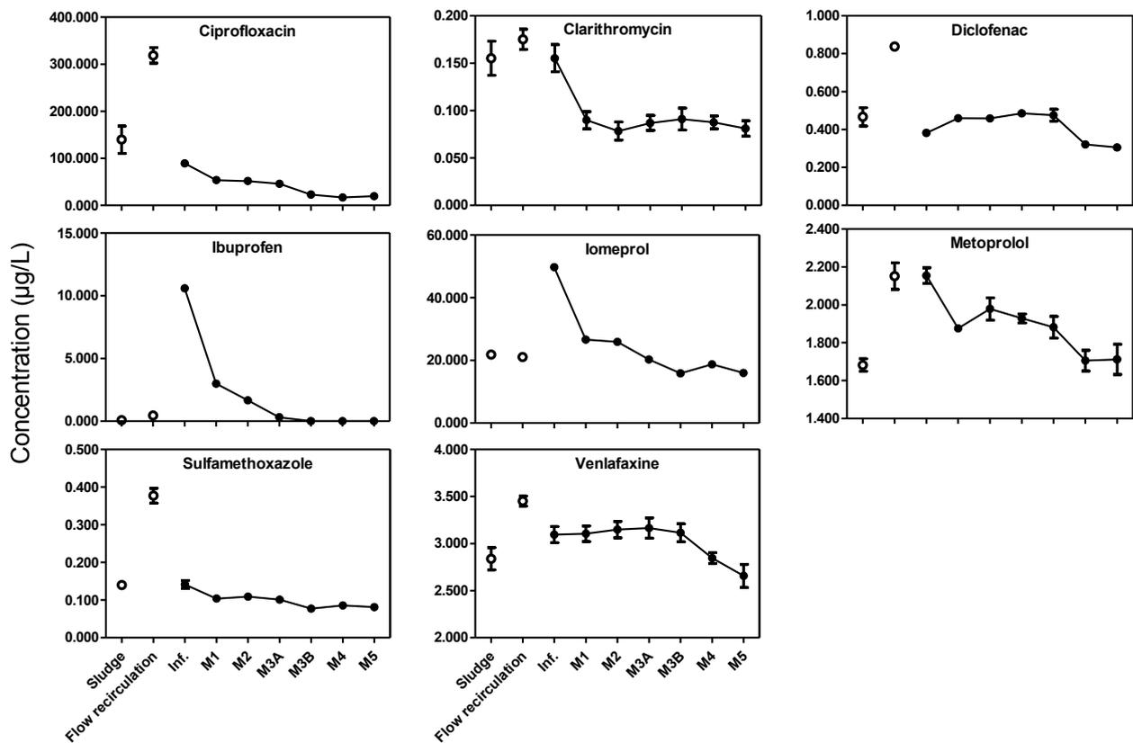
**Figure 46. Average concentrations and SD (n=3, each sample was analyzed twice) in the HYBAS™ pilot reactors during the continuous flow experiment. The impact on pharmaceutical concentration was measured as recirculation concentration and sludge.**
