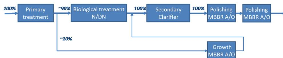
**Figure 60. MBBR Alternating Operation incorporated in typical municipal WWTP scheme.**
