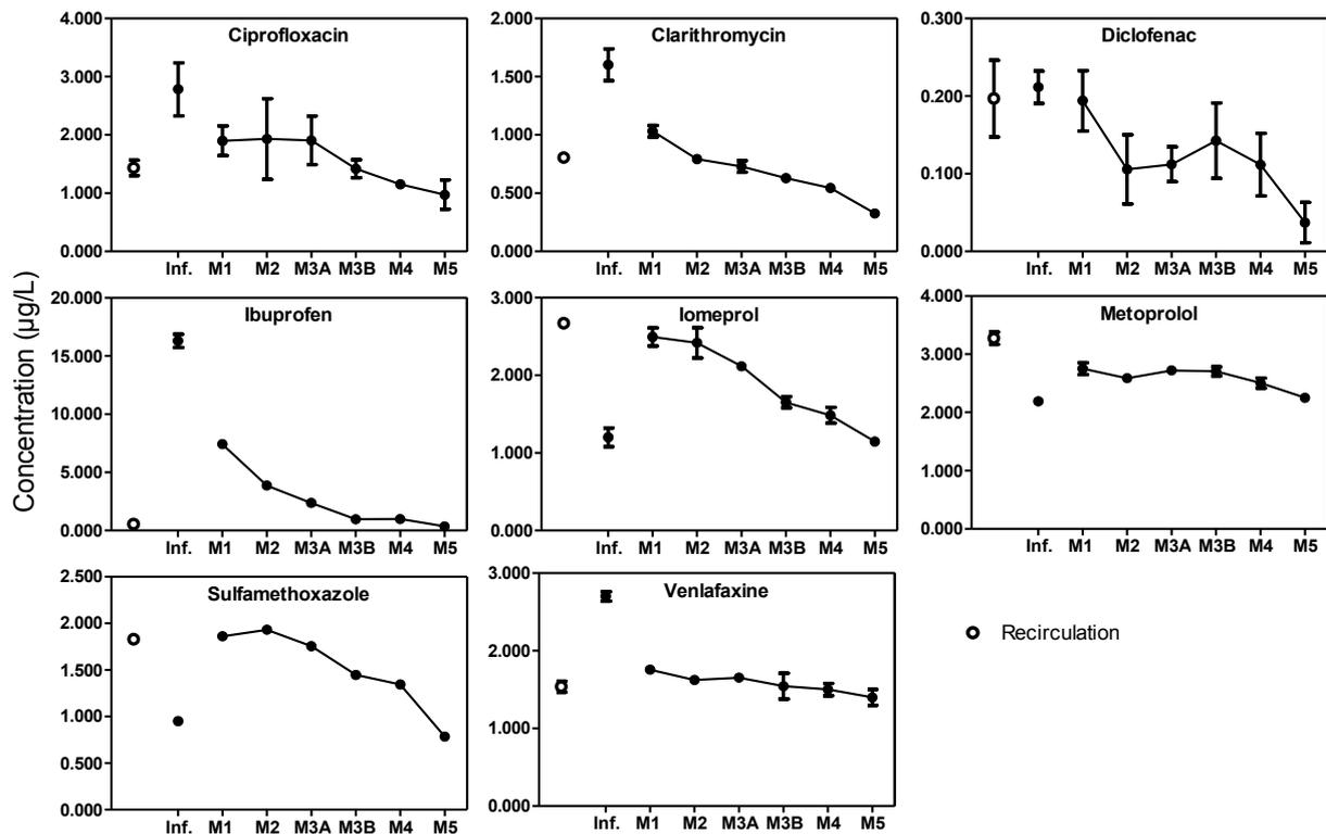
**Figure 33. Average concentrations and standard deviations (n=3, each sample was analyzed twice) in the different MBBR reactors during the continuous flow experiment. The impact on pharmaceutical concentration was measured as recirculation concentration in which concentrations in M1 include both recirculated wastewater from M3B and influent (inf.).**
