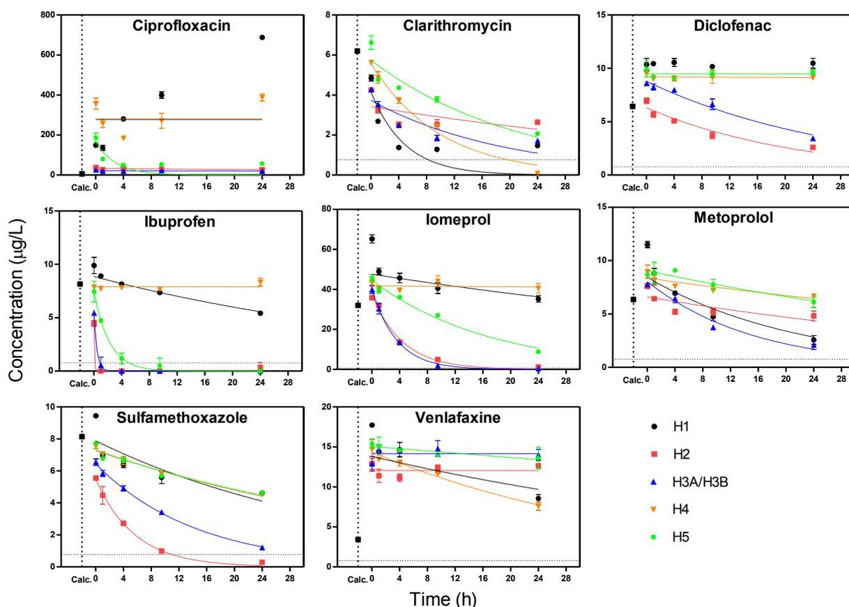
**Figure 44. Concentrations of selected pharmaceuticals during batch experiment in each reactor (H1, H2, H3, H4 and H5). Filled lines correspond to a first-order kinetics fitting. Black squares are theoretically calculated dosages of each compound based on added stock solution. Dashed lines represent LOQ.**
