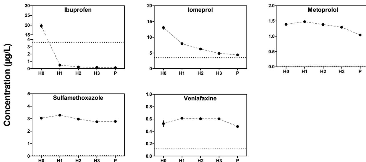
**Figure 14. Overview of the concentration of the selected pharmaceuticals through the HYBAS™ with polishing, (due to analytical complications and detection of indigenous concentration below LOQ, 5 out of 8 compounds were shown).**
