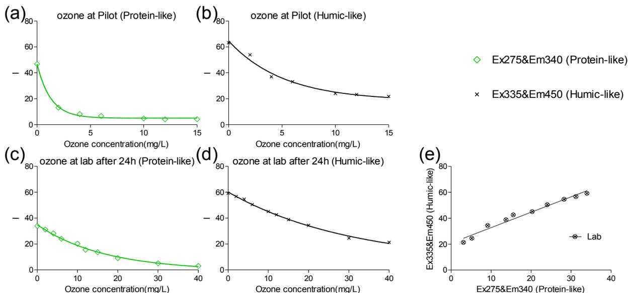
**Figure 37. Comparison of remaining natural fluorescence of M5 effluent treated by ozone using the pilot or bench method. The correlation of the two fluorescence wavelengths ( $\lambda_{275, 340}$ ) and ( $\lambda_{335, 450}$ ) was fitted by a straight line so correlations between lab scale and pilot-scale experiments were possible.**
