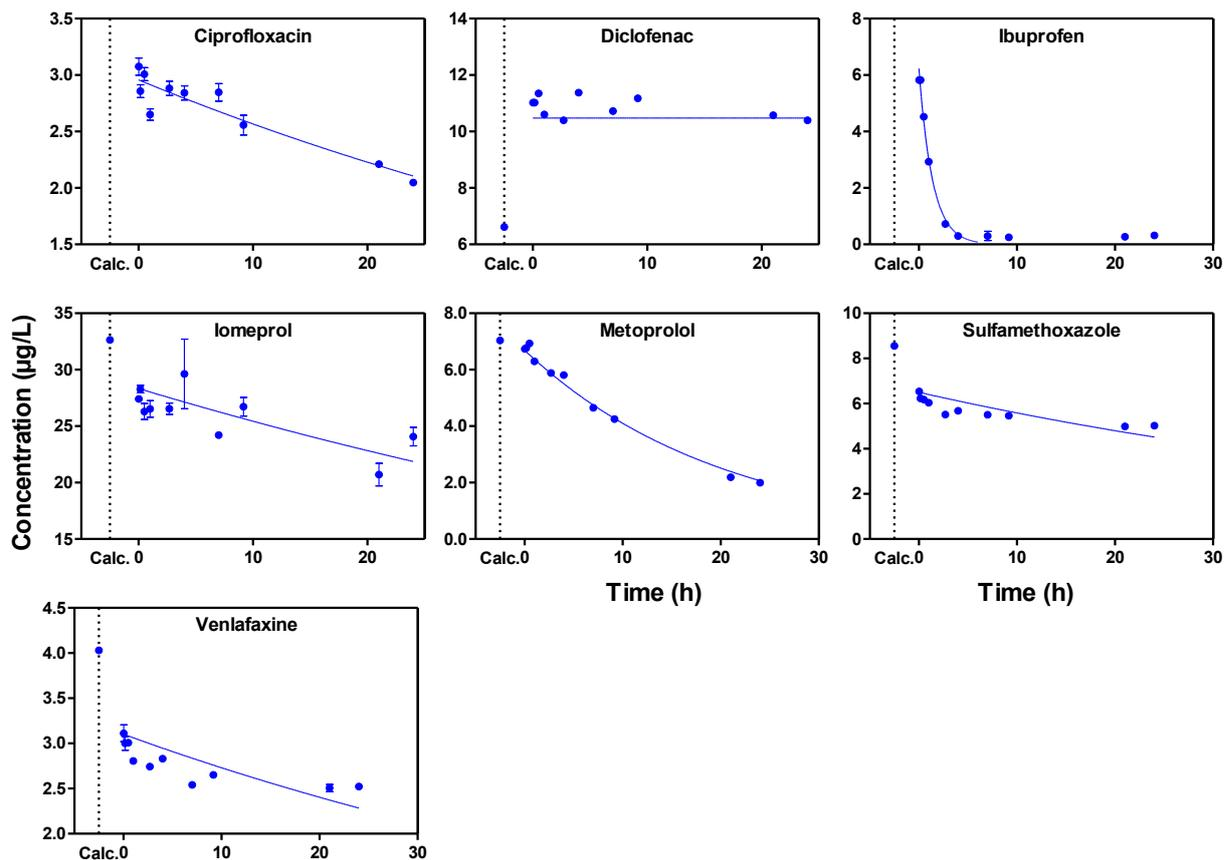
**Figure 13. Concentration of selected pharmaceuticals in CAS in the batch experiment. Filled lines correspond to a first-order kinetics fitting while concentrations shown on the vertical dotted-line denote the theoretical concentration based on spiking. Due to analytical complications, clarithromycin was not shown.**
