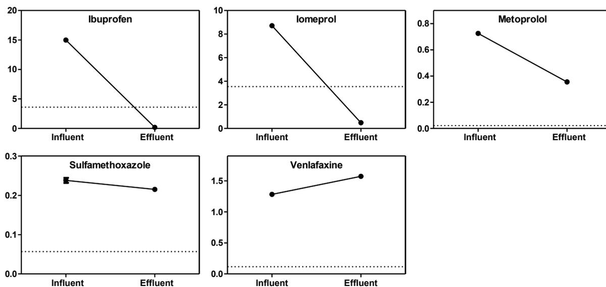
**Figure 15. Overview of the concentration of the selected pharmaceuticals in CAS. The dotted line indicates LOQ, (due to analytical complications and detection of indigenous concentration below LOQ, only 5 out of 8 compounds were shown).**
