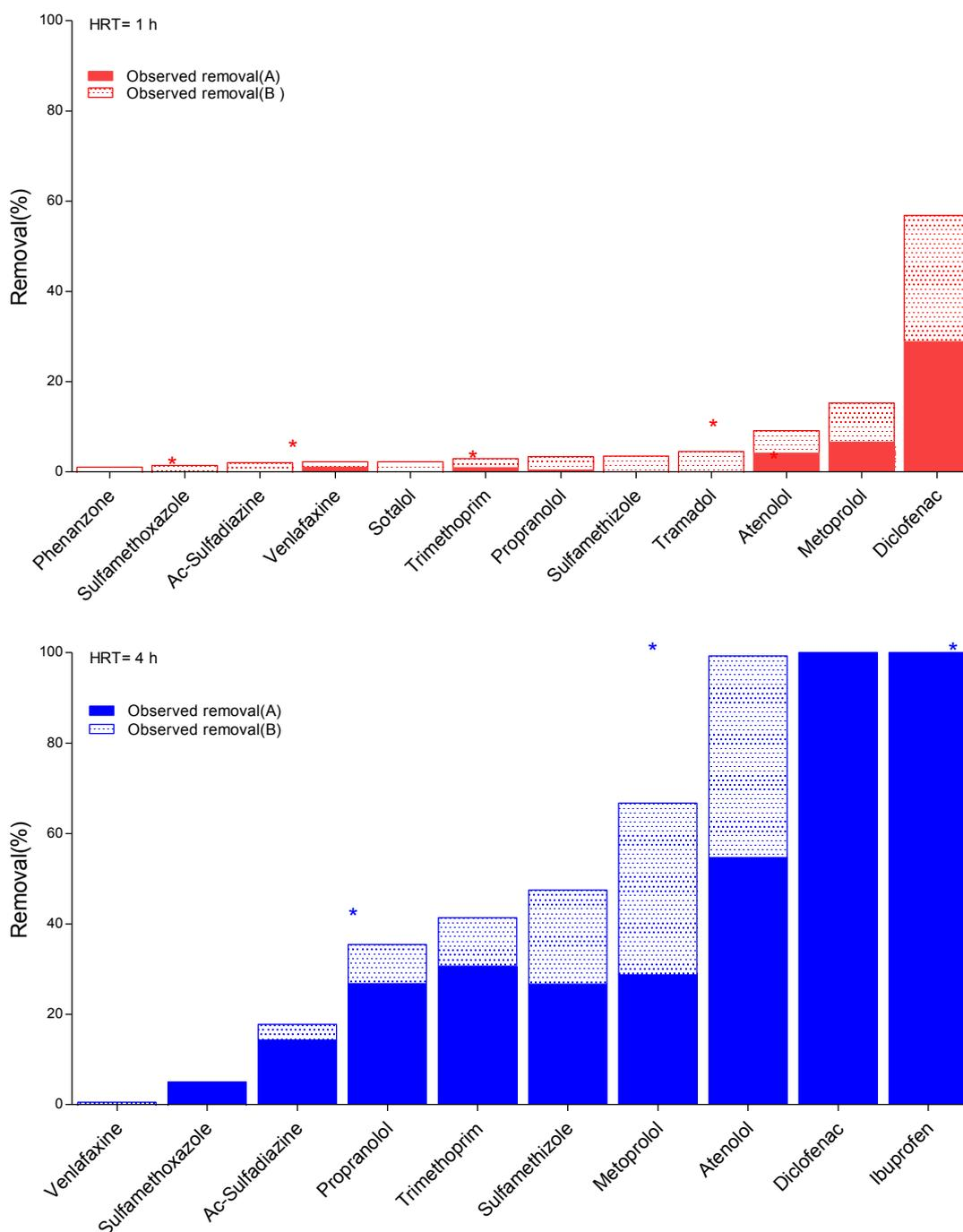
**Figure 22. Measured removal from the continuous flow experiments at two different HRT (1 h and 4 h) over the polishing reactors (position A and B), shown as percentage degradation. A star indicates that compound concentration was below LOQ.**
