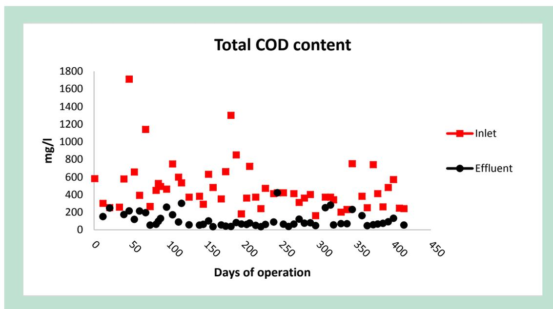
**Figure 9.** The content of COD in un-filtrated inlet- and effluent samples of the HYBAS™ bench-scale plant.
