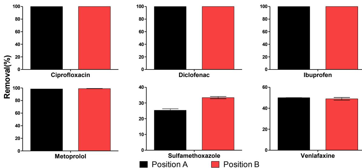
**Figure 20. Potential capacity of the two positions, for removal pharmaceuticals over a period of 24 hours. Position A is fed from effluent waters, and position B from the effluent of position A, (due to analytical complications, e.g. a shift in the retention time, clarithromycin and iomeprol were left out).**
