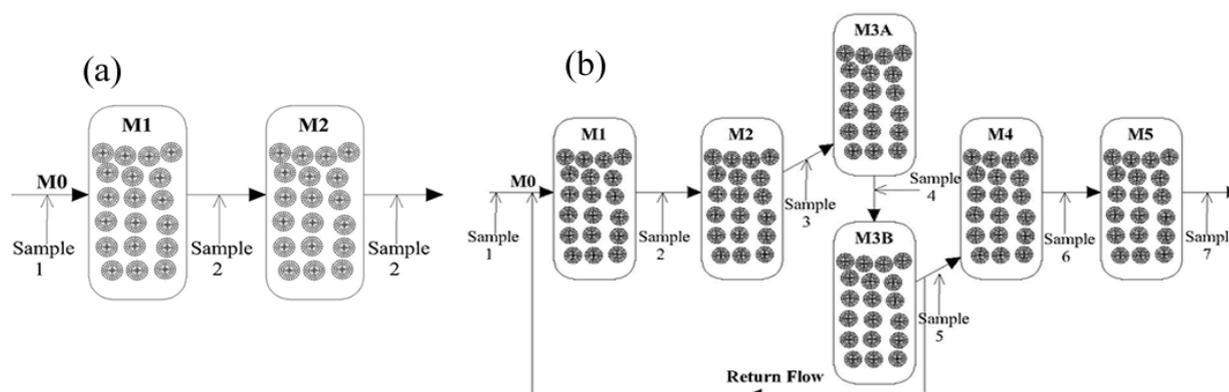
**Figure 6. Overview of the experimental setup for determining the actual capacity of the treatment technology, investigated in the corresponding treatment scale ((a): lab-scale sampling; (b): pilot-scale sampling). Samplings between the reactors are carried out based on the HRT of the system.**
