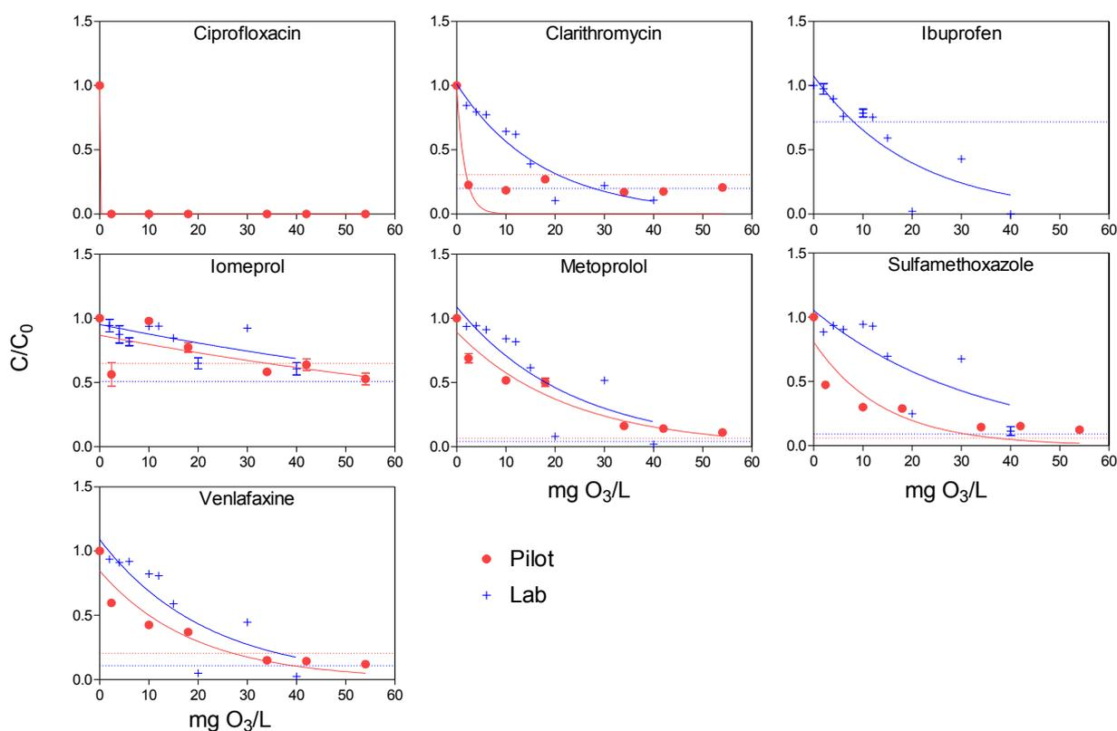
**Figure 36. Pharmaceutical removal by ozonation in the effluent of the staged MBBR pilot plant using either the onsite continuous pilot ozonation system or batch treatment in bench scale. Dashed lines correspond to limit of quantification (LOQ) by HPLC-MS/MS for each experiment. Error bars represent standard deviations.**
