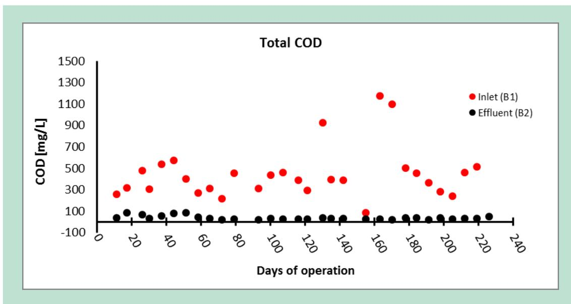
**Figure 39. Overview of total COD content in inlet and effluent samples during HYBAS™ pilot plant operation.**
