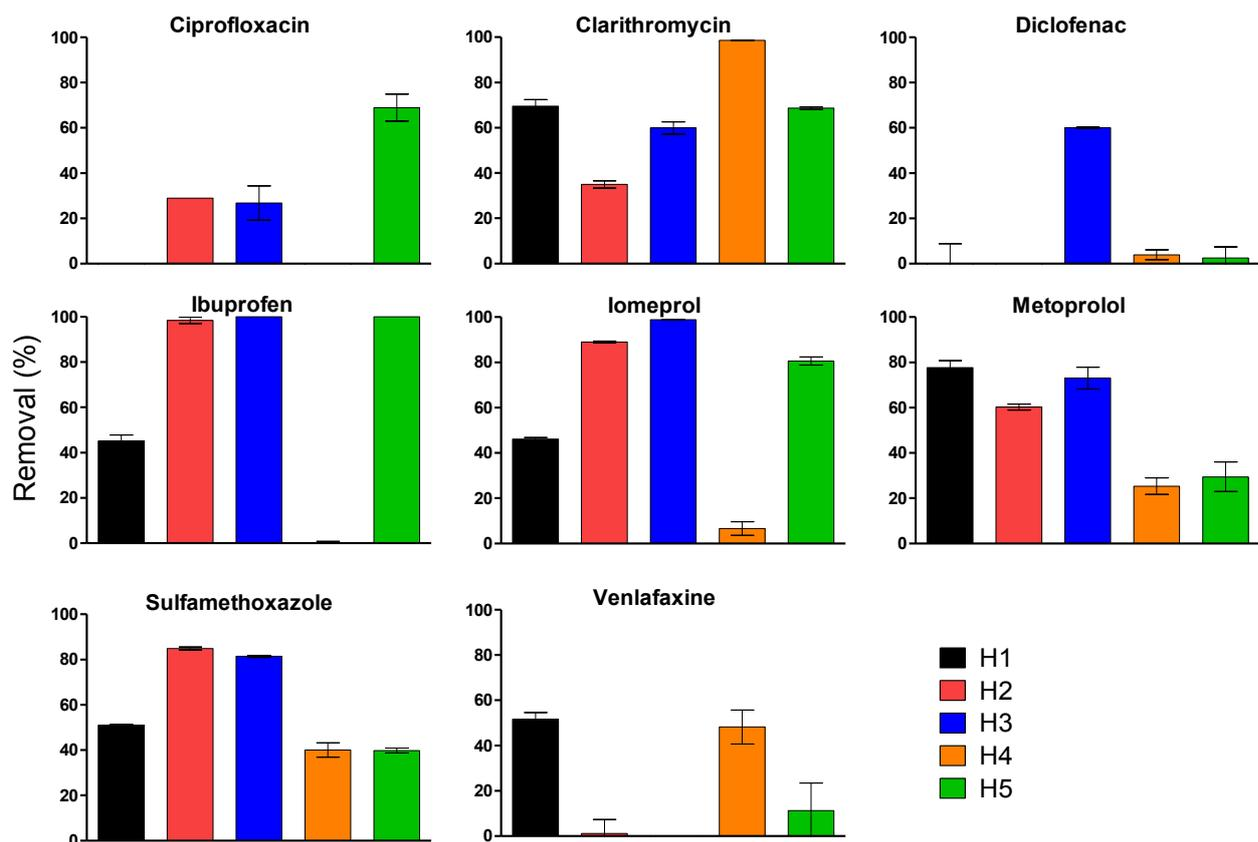
**Figure 45.** The potential capacity (%) of each reactor to remove pharmaceuticals over a period of 24 hours. Reactors H1 and H4 were denitrifying (black and orange) where the remaining reactors were aerobic. Carriers were present in H3, H4 and H5.
