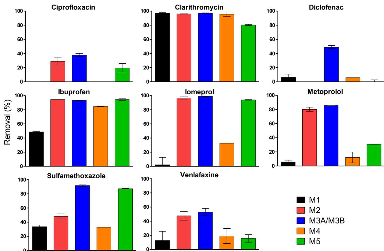
**Figure 32. The potential capability of each reactor to remove pharmaceuticals over a period of 24 hours. Reactors M1 and M4 (black and orange) were denitrifying whereas the remaining reactors were aerobic.**
