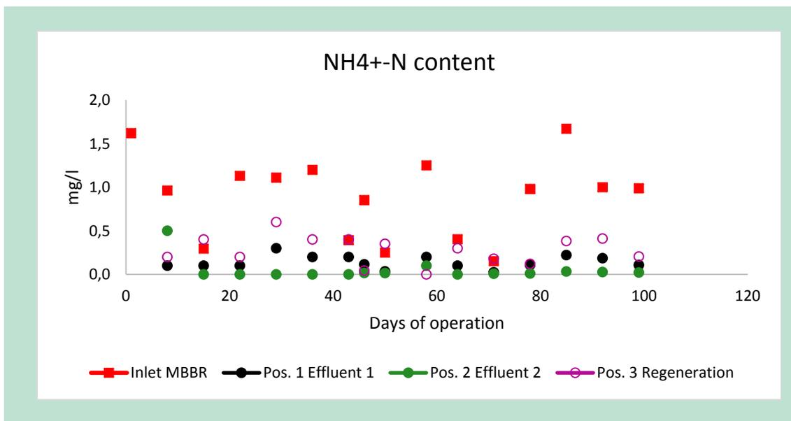
**Figure 18. Ammonia content of inlet MBBR and of the different MBBR reactor positions (A, B and C).**
