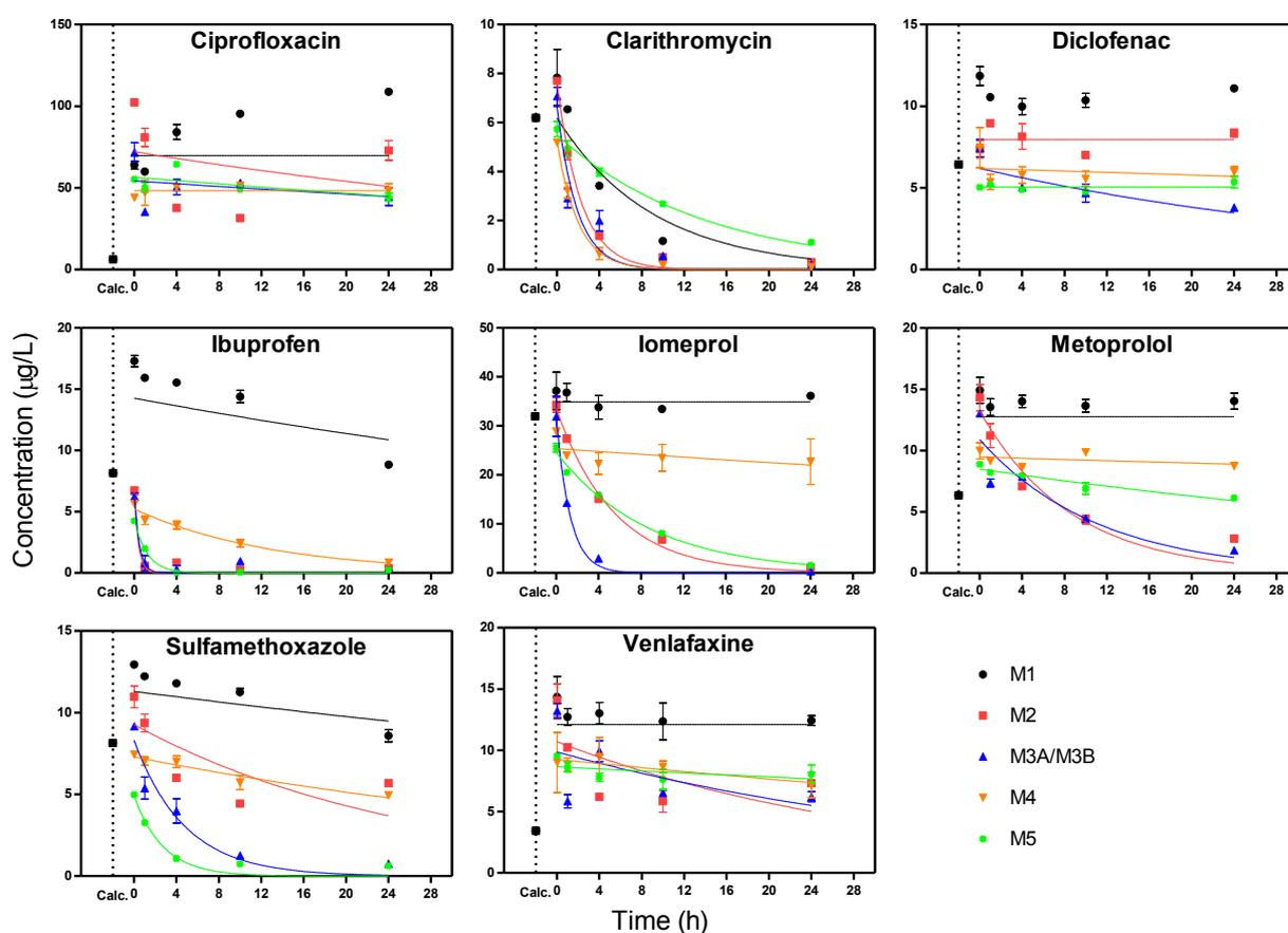
**Figure 31. Concentrations of selected pharmaceuticals during spiking batch experiment in each reactor (M1, M2, M3A/M3B, M4 and M5). Filled lines correspond to a first-order kinetics fitting. M 1 and M4 are denitrifying, the remaining reactors are aerobic. Black closed square symbols in the figure denotes the theoretical calculation of individual pharmaceutical concentrations according to stock concentrations of pharmaceuticals.**
