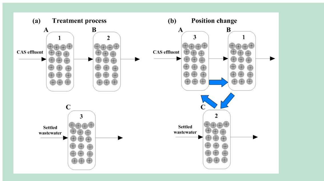
**Figure 2. Operation of two MBBR tanks polishing effluent from the Viby WWTP (positions A and B), while the growth/regeneration of biofilm was stimulated in a third MBBR reactor (position C).**
